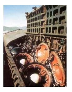
Torpedo munitions comprised 24 torpedoes held in open rack magazines, potentially including torpedoes of nuclear capability, firing from 2x650mm and 4x533mm torpedo tubes in the bow (No 1) compartment. The armaments could also include ASW Harpoontype rockets and seabed mines also deployed from the forward torpedo tubes.
